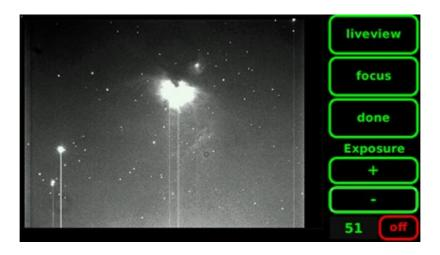
The Find and Focus tool is used to frame the desired sky view and/or to adjust focus.
