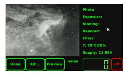
The **Monitor** tool can be used to follow or interrupt the photo sequence currently in progress. It provides the following information related to the current exposure:
