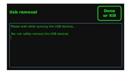
The USB removal tool is used to allow a safe removal of USB storages connected to the camera. Any connected device is available in the usb subdirectory in the main photos directory. The USB removal script is launched when pressing the button on the desktop. Touch Done or Kill to come back to the desktop after script execution or to kill the task if it gets locked.
