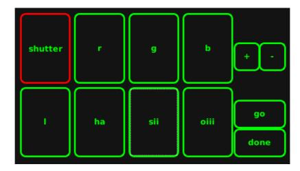
The Filterwheel tool is used to control, where available, the integrated filter wheel, to select a filter for the Find and focus tool.
