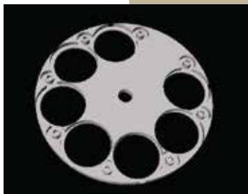
The AST8300 incorporates an internal seven position filter-wheel. The filter-wheel accepts standard unmounted 27mm filters. The eighth position of the filter-wheel is occupied by the shutter. The exact position of the filter-wheel is controlled through an optical sensor.
