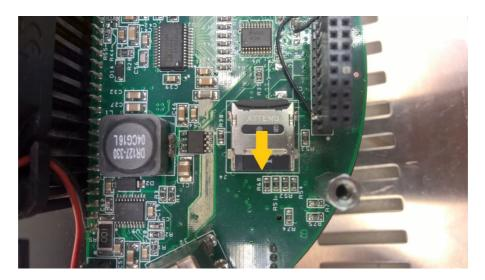
6) When unlocked the uSD slot cover can be opened
