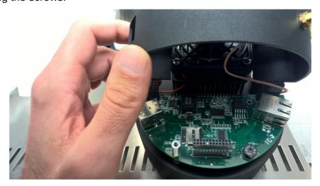
5) Unlock the uSD slot sliding its cover as indicated by the arrow in the picture
