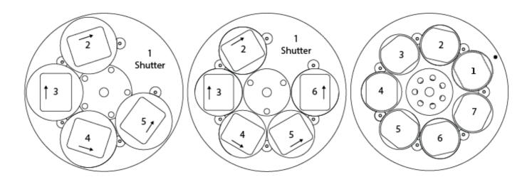
At the beginning of the exposure, the 4F and 5F wheels move CW or CCW depending on which filter is selected in order to minimize filter crossing to reach the selected one (see the arrows), while the 7F always move in the same direction as the shutter is not in a fixed position.
