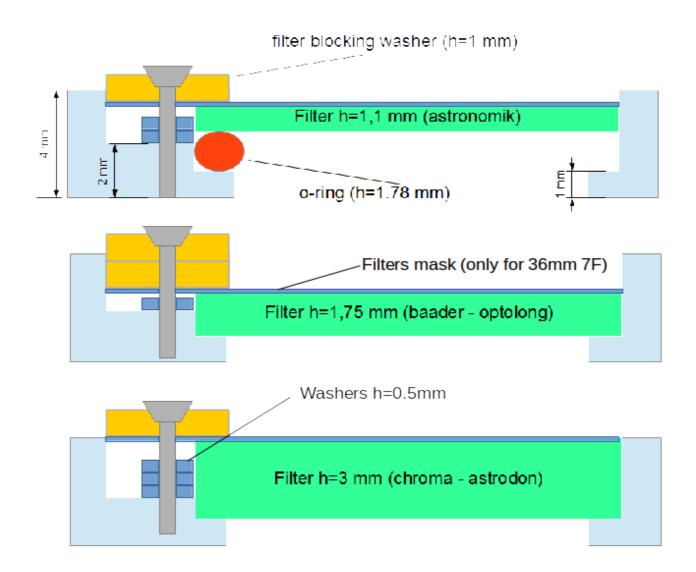
9. insert the o-ring where needed (only for thin filters of 1.1 mm thickness)
