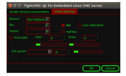
It is necessary to specify the guider device you will work with. To do this, you should choose it from the 'Device' list. Every time you change guider it is necessary to restart the program for the connection to the specified device to occur.
