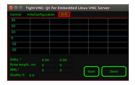
Press 'Start' to begin guiding. The drift graph, current values of corrections and statistics are updated at every new image from the guider. When ready, you can close the guiding application by pressing 'Done'. Of course guiding will continue in background and you can get back to the 'Drift' tab by simply clicking on the autoguider icon on the camera desktop.
