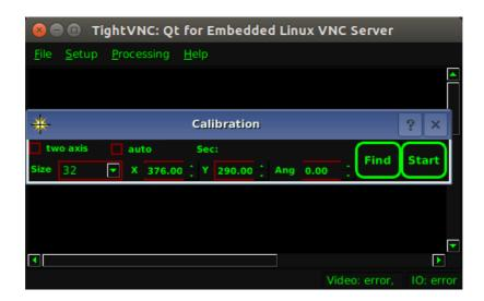
Use the 'two axes' parameter to choose the two-axes or one-axis calibration. If the polar axis is aligned, it is recommended to use the automatic mode of calibration - parameter 'auto mode'.
