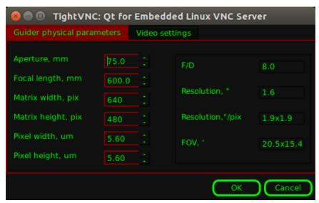
When the video device and the telescope mount control device are connected and working in the program, you must specify several parameters before the guiding can be started:
