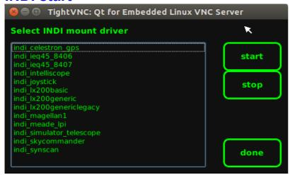
The INDI start app is used to start and stop INDI drivers. At the moment only mount drivers are supported and used by the GoTo and Find and Focus apps. In particular, the GoTo app can't be started if the INDI driver corresponding to your mount is not started.
