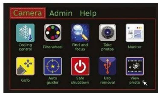
▲ The camera is controlled by a set of internal applications – these cover everything from cooling to image capture
